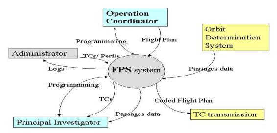
Figure 2: Flight Plan Supporting System Interfaces
