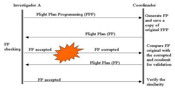
Figure 6: Sequence Diagram for a Test Case
