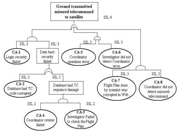
Figure 3: Fault Tree Analysis (FTA) for Flight Plan Supporting System
